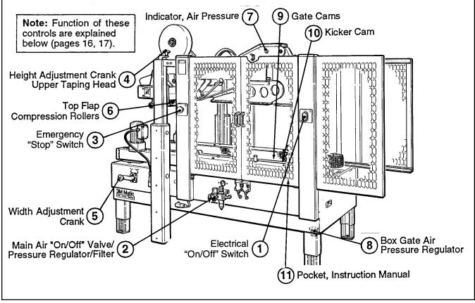
Figure 3-2 – Controls, Valves and Switches
